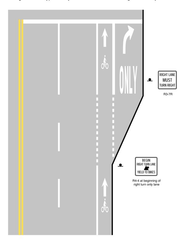
Figure 9C-4. Typical Bicycle Lane Treatment at Parking Lane into a Right Turn Only Lane
