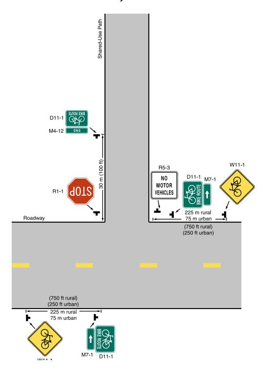
Figure 9B-3. Typical Signs and Markings for Shared-Use Paths
